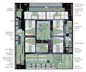
memory capacity powered by dual interleaved DDR3 DRAM memory interfaces, and high I/O throughput based on serializer/deserializer (SerDes) high-speed links. The RAD5545 SoC microprocessor singlehandedly replaces multiple cards of previous generations with four RAD5500™ 32/64-bit Power Architecture processor cores, three levels of on-die cache, four RapidIO® (SRIO) ports, and a 16-port SpaceWire router.
